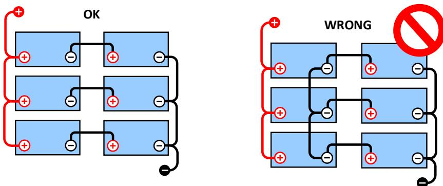
Due to the voltage drop over the positive and the negative cables the midpoint voltage are not identical.
