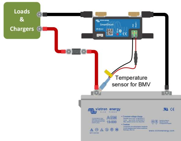
Please note that if the temperature sensor is used, the red power cables that came with the SmartShunt are not needed. The temperature sensor will replace these cables.
