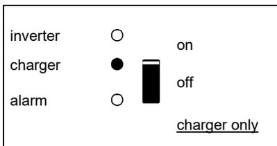
The AC input voltage is switched through and the charger operates in bulk or absorption mode.
