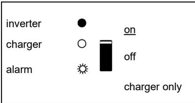
The inverter is switched on and supplies power to the load.
