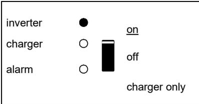
The inverter is switched on and supplies power to the load. Battery operation.
