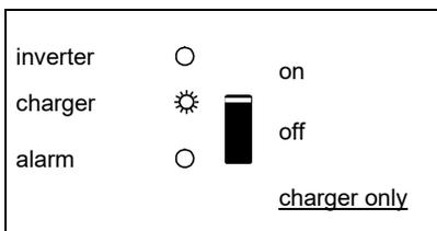
The AC input voltage is switched through and the charger operates in float mode.
