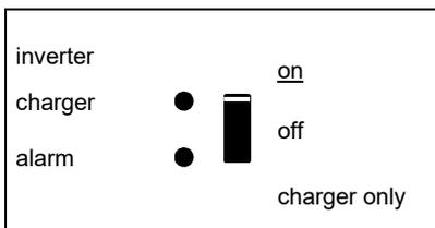
The AC input voltage is switched through and the charger is switched off. The battery charger can not reach battery end voltage (bulk protection mode).
