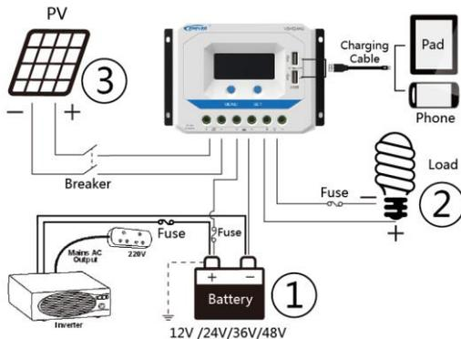
Figure 2 Connection diagram
