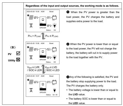
Note: When the battery voltage is greater than or equal to the LVR value, or the battery SOC is greater than or equal to the LER value, the working mode returns to state 2.
