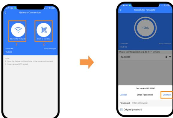
**Step4:** Connect the WiFi terminal to the 2.4G WiFi network by searching for the hotspots or scanning the QR code.
