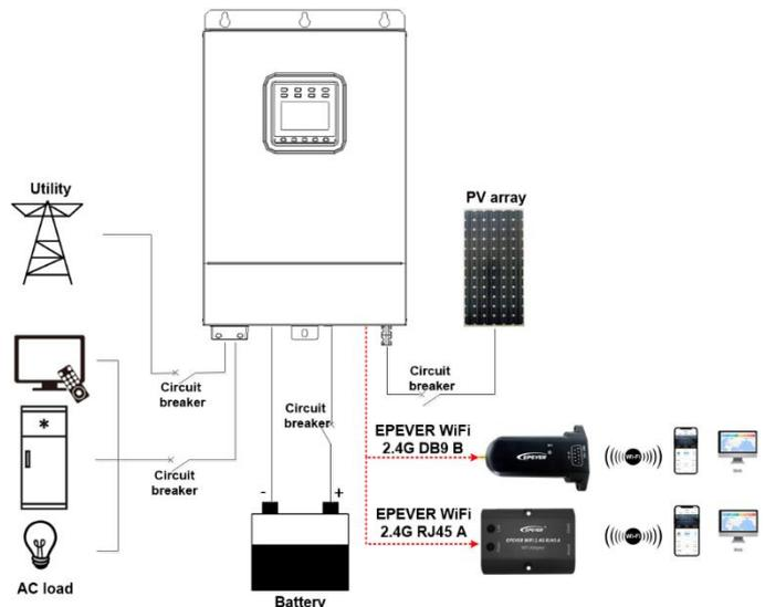
**Note:** EPEVER WiFi 2.4G RJ45 A is suitable for the controller, inverter, or inverter/charger designed with an RJ45 port. EPEVER WiFi 2.4G DB9 B is ideal for the device designed with a DB9 interface. For detailed connection cables, refer to the connected device's accessories list.
