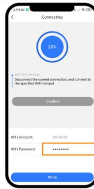
**Step6:** Input the WiFi password, and click the "Write" to connect the WiFi network.
